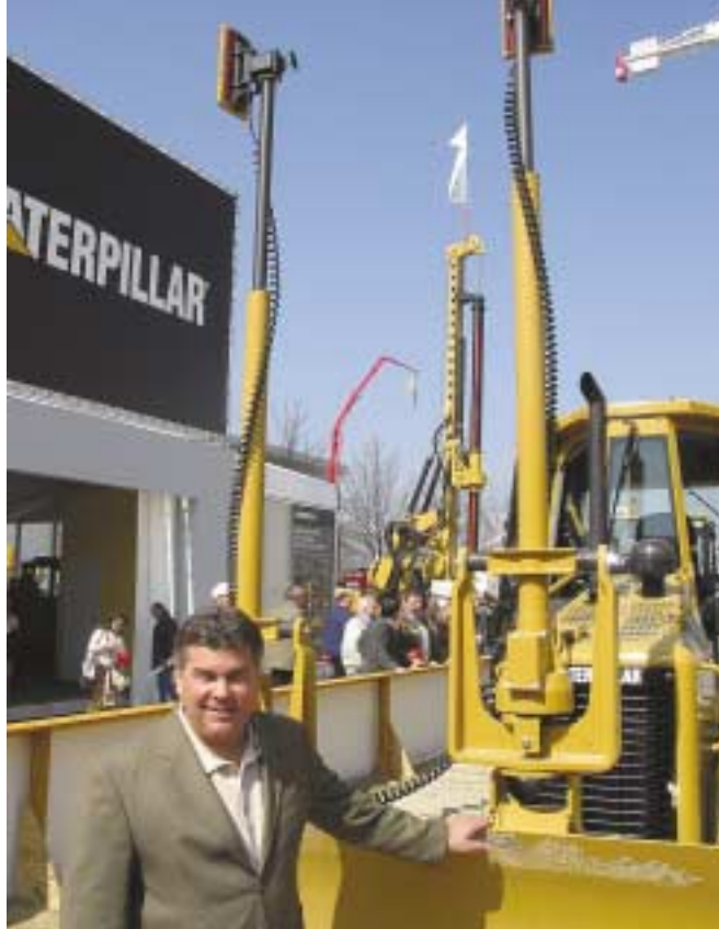
Dave Pinaire heads up the machine control division of Cat — seen at BAUMA introducing AccuGrade on a D5. Note laser receivers on telescopic masts.
