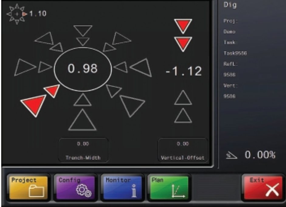
Above: Screen display of Leica Geosystem's Digger 3D is simplicity itself. Large graphic on the left shows horizontal direction to move the bucket to comply with onboard computer design of the task—at right, vertical direction. Below: Graham Wirth, Leica Geosystem's business development manager for machine control (Asia), with Adam Forsyth, Digger 3D product manager, and Stefan Meulen, (in the excavator cab), in-house applications engineer.
