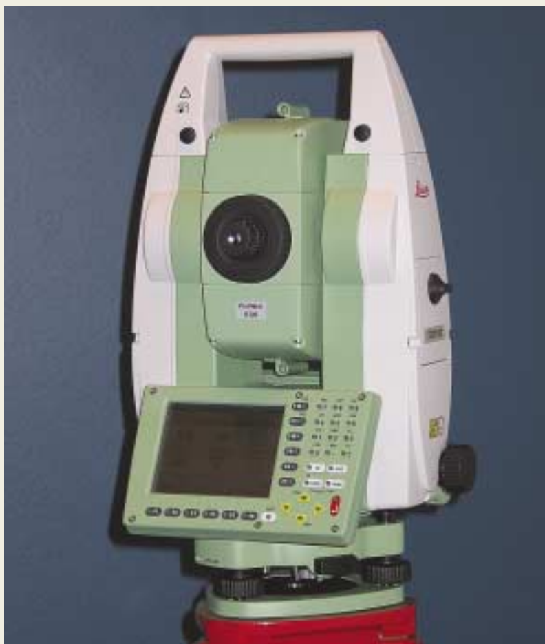
The entry-level version of Leica’s new TPS1200 total station is remarkably inexpensive considering its excellent performance. The operating platform is identical to the GPS1200 (below), so learning the ropes on one means knowing how to operate both.
