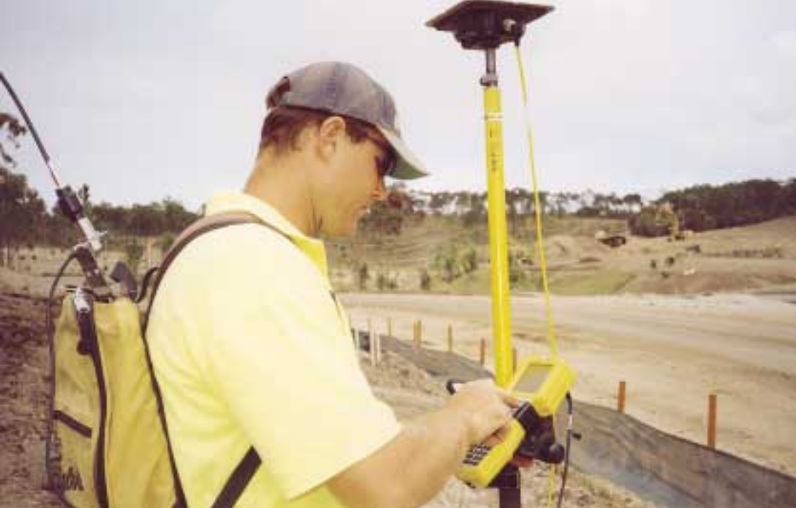
Left: using data received five minutes earlier over his mobile phone, Steve establishes the position of the next hydrant while the line is being laid. Above: close-up of Trimble GPS rover model 4700 Below: picking up location of a silt fence for inclusion in progress claim.
