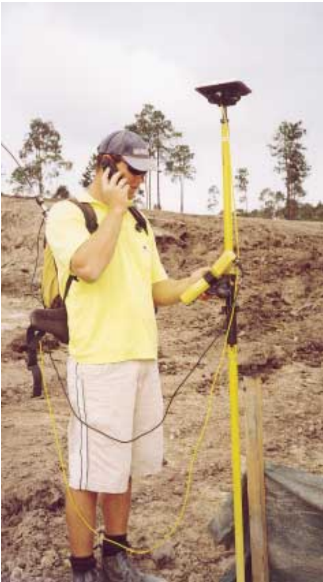
Left: using data received five minutes earlier over his mobile phone, Steve establishes the position of the next hydrant while the line is being laid. Above: close-up of Trimble GPS rover model 4700 Below: picking up location of a silt fence for inclusion in progress claim.
