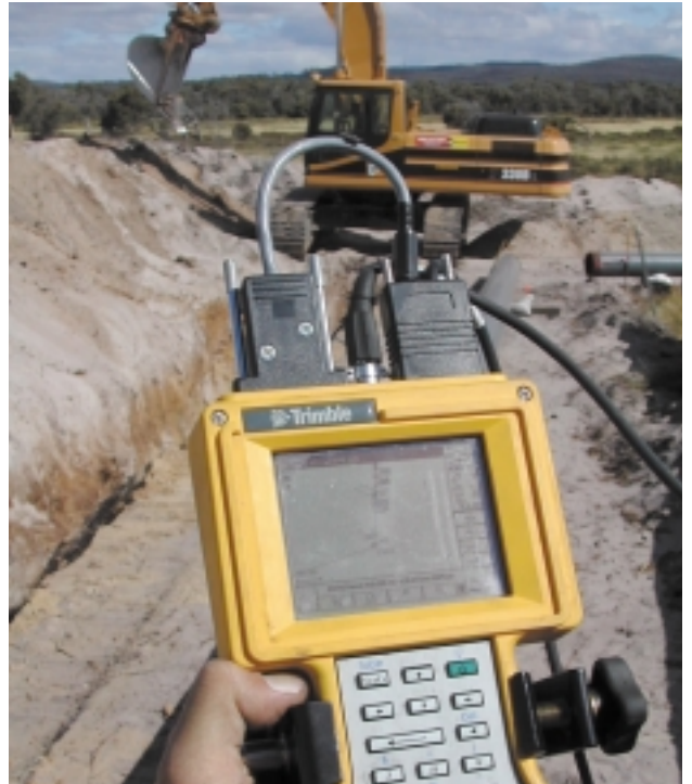
Australia's largest GPS application at present involves twelve RTK rovers on a $400 million gas pipeline connecting Tasmania with Victoria.
