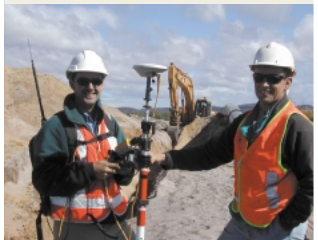
Australia's largest GPS application at present involves twelve RTK rovers on a $400 million gas pipeline connecting Tasmania with Victoria.
